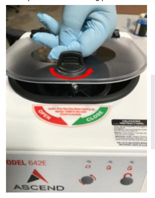
After a run has completed, the unit will gradually slow down and come to a stop. (This can take a minute or two.) When it does, rotate the latch release knob counterclockwise to the "horizontal" position, and lift the lid open.
