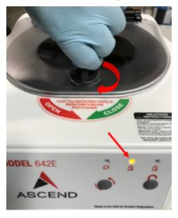
There will be a slight "click" when the locking mechanism is in the "locked" position, and the yellow "locked" light will illuminate.
