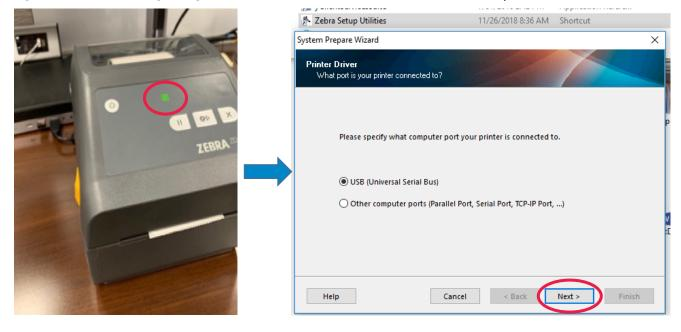
Your printer should appear as installed now on Zebra Set-up Utilities.
