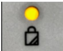
The light indicates that the lid is closed and the locking mechanism is locked.
