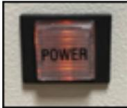
Button glows orange when the unit is powered on.
