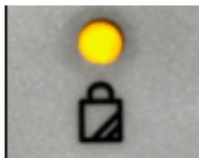
The light indicates that the lid is closed and the locking mechanism is locked.
